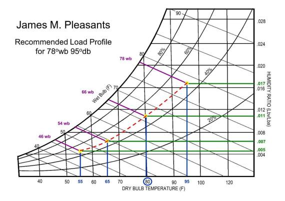
Notice the dry bulb design points shown in blue on the horizontal axis of the psychrometric chart. To determine wet bulb temperatures at these design points, follow the (blue) vertical line from these four dry bulb values up to the curved (dotted red) line that represents a constant 47% relative humidity. From that point follow the purple diagonal line to the left where you find the wet bulb temperature that corresponds with these conditions:
